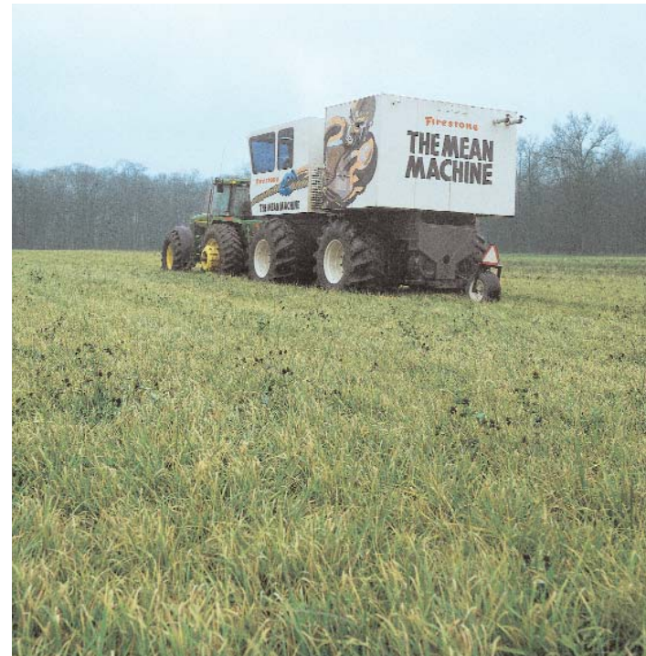
The Firestone Mean Machine, below, tests agricultural tires at the company's test facility in Columbiana, Ohio.
